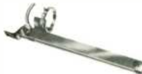
SPRING HANGER. ANDREW 13925. Use at 10 ft. intervals. Accommodates line expansion. Mounts through \frac{3}{16} " diameter hole or adaptors. Part No. 097 6122 000
