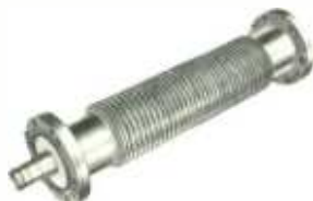
FLEXIBLE SECTION. ANDREW 19209B. Accommodates vibration and angles up to 30 degrees. Maximum offset is \frac{1}{2} ". Length, 18". Part No. 099 0441 000
